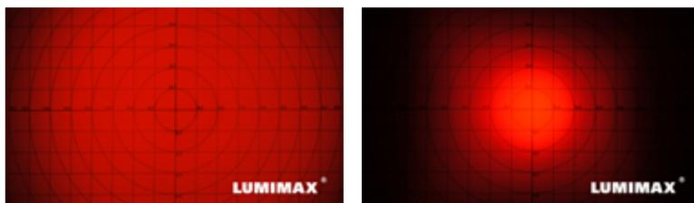
High Power Lighting: left with 49° lenses, right with 10° lenses (at a working distance of 1.5 m)
