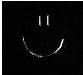
Scratch on acrylic glass – dark field backlight
