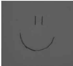
Scratch on acrylic glass – diffuse backlight
