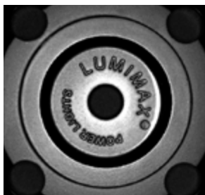
Conventional image capture using LED ring lighting
