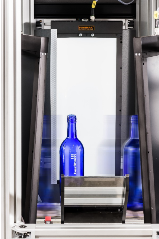
Photo 2 Thanks to collimated Area Lighting solutions from LUMIMAX®, edges and production defects are shown clearly on the object image
